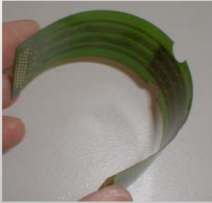
~0.008" thick film conformable to curved surface
