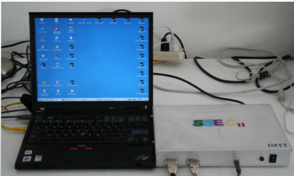
SSEC II-B is connected to a laptop through a UBS cable
