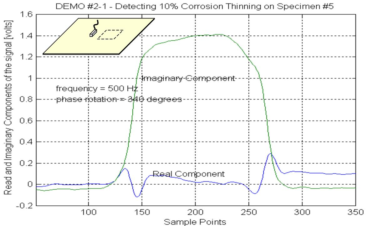
Figure 4. DEMO #2-1 - Thickness = 0.063", Corrosion Depth = 0.006", Relative Depth = 10 %
