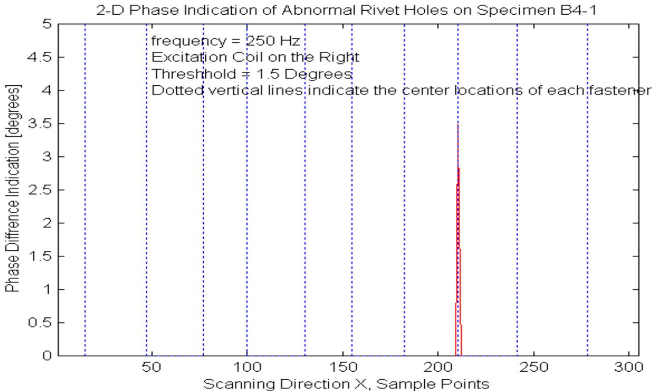
Figure 13. DEMO #4 - Total thickness = 0.446", Crack length = 0.031", Crack location - bottom surface of 2<sup>nd</sup> layer (The cracked hole is identified by its phase angle derivation)
