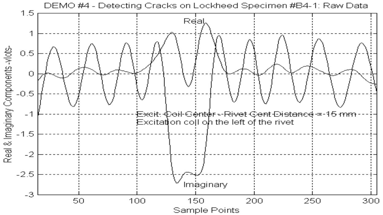
Figure 10. DEMO #4 - Total thickness = 0.446", Crack length = 0.031", Crack location - bottom surface of 2<sup>nd</sup> layer (Raw Data)
