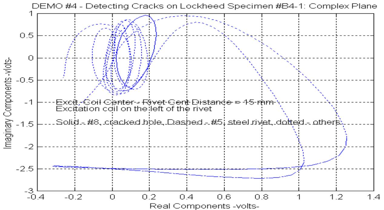
Figure 11. DEMO #4 - Total thickness = 0.446", Crack length = 0.031", Crack location - bottom surface of 2<sup>nd</sup> layer (Complex Plane)
