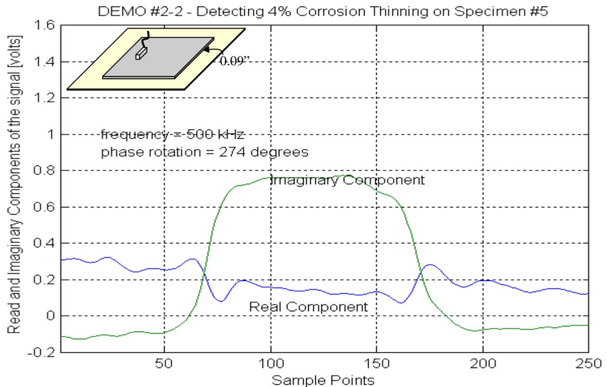
Figure 5. DEMO #2-2 - Thickness = 0.153", Corrosion Depth = 0.006", Relative Depth = 4 %
