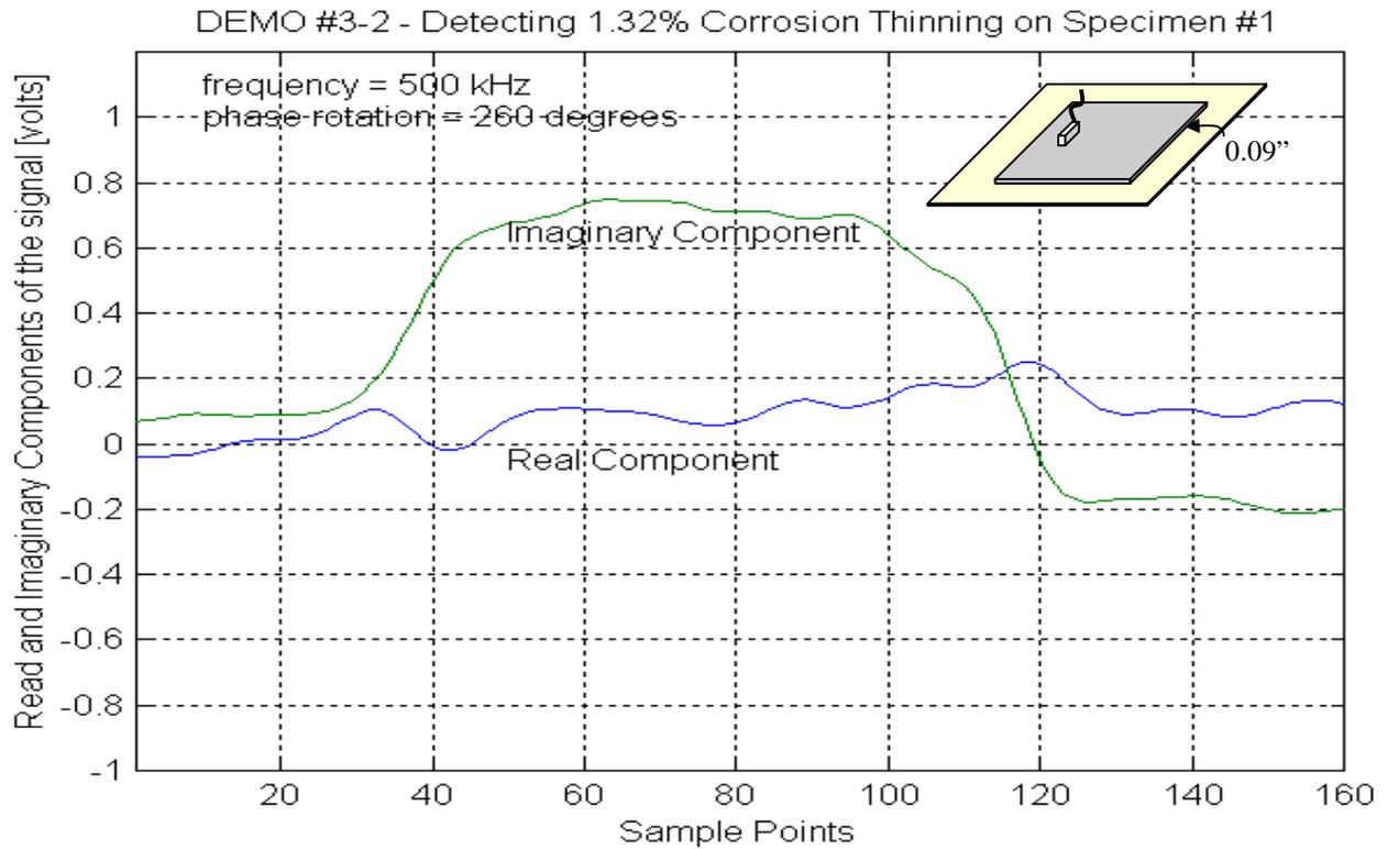
Figure 8. DEMO #3-2 - Thickness = 0.153", Corrosion Depth = 0.002", Relative Depth = 1.32 %
