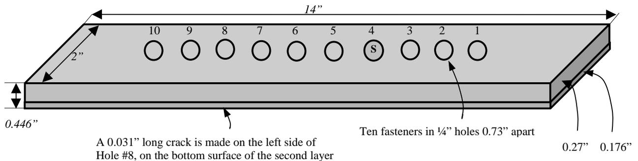
Figure 2. A typical Lockheed Georgia Specimen of Group B: Specimen #B4-1:
