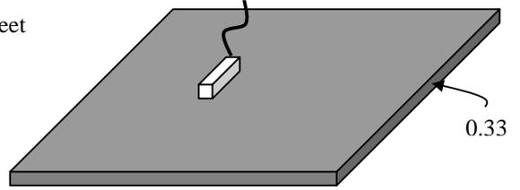
B. DEMO#1-2 Scanning on a 0.33" aluminum sheet with a discontinuity below
