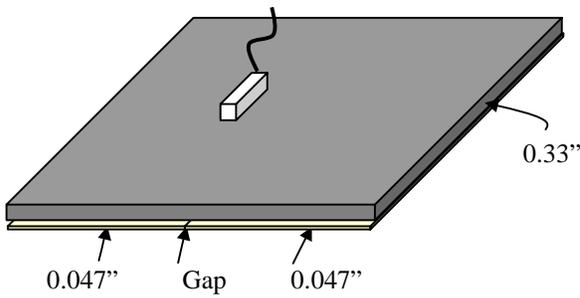
C. DEMO#1-3 Add a 0.182" thick plate to make total thickness to be 0.51"
