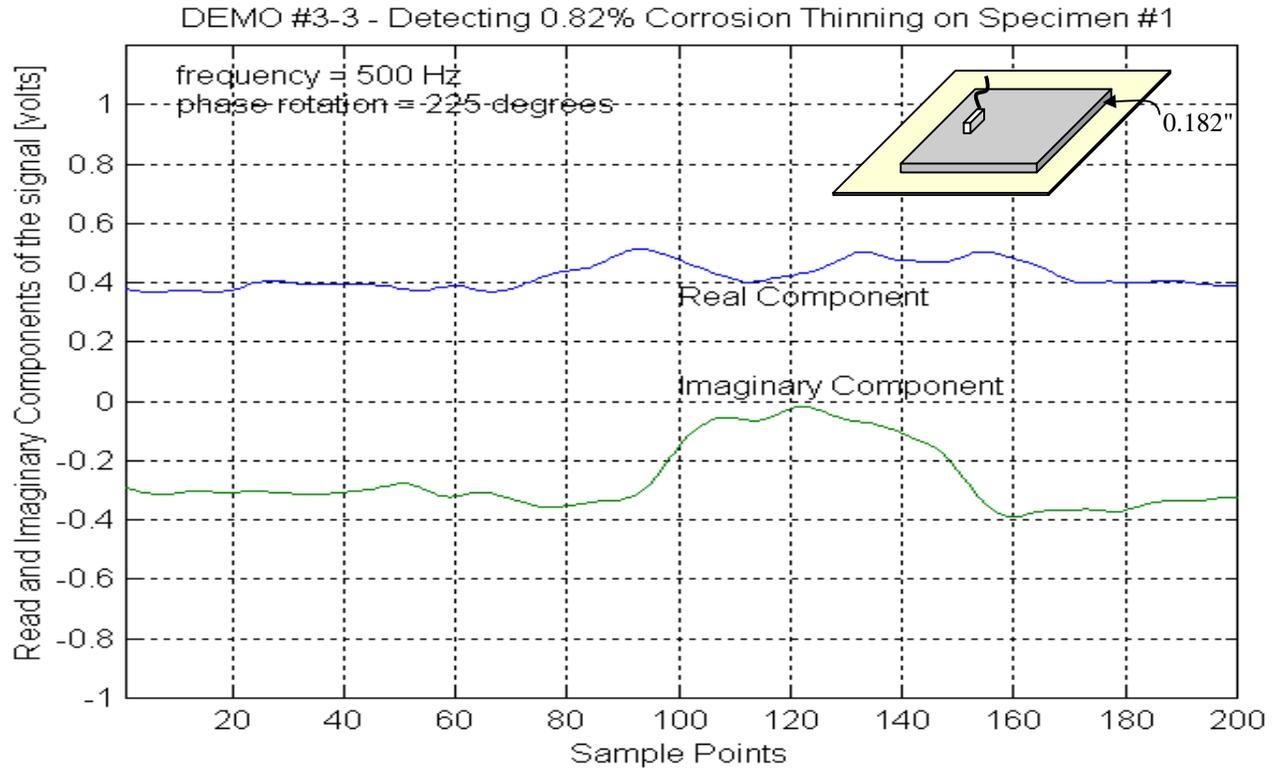
Figure 9. DEMO #3-3 - Thickness = 0.245", Corrosion Depth = 0.002", Relative Depth = 0.82 %
