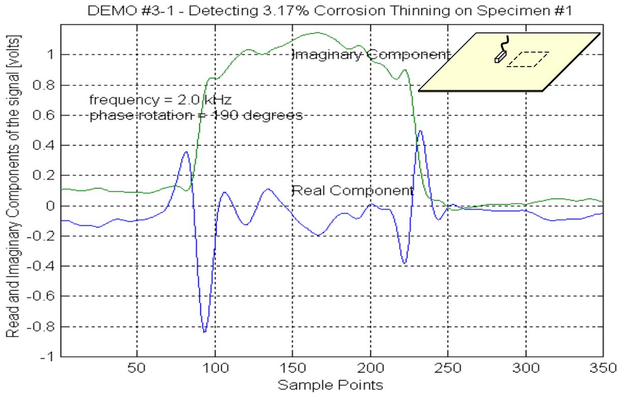
Figure 7. DEMO #3-1 - Thickness = 0.063", Corrosion Depth = 0.002", Relative Depth = 3.17 %
