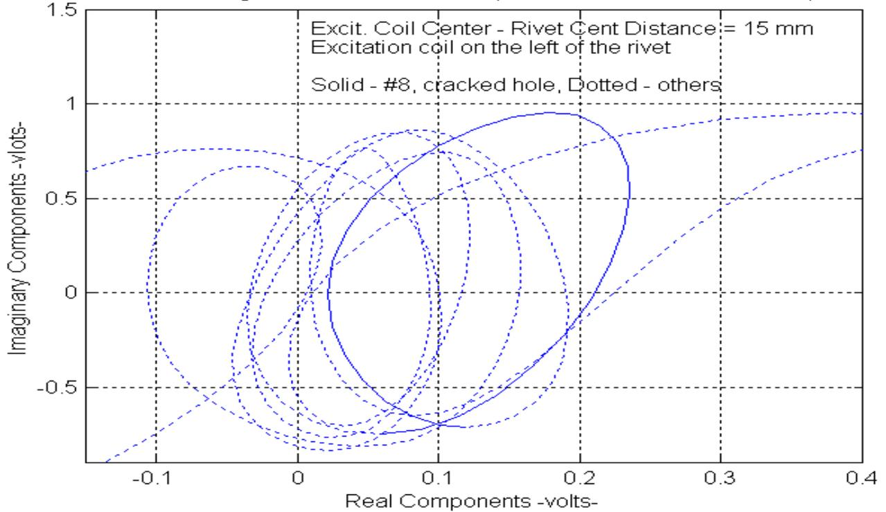
Figure 12. DEMO #4 - Total thickness = 0.446", Crack length = 0.031", Crack location - bottom surface of 2<sup>nd</sup> layer (Zoom-In Complex Plane)
