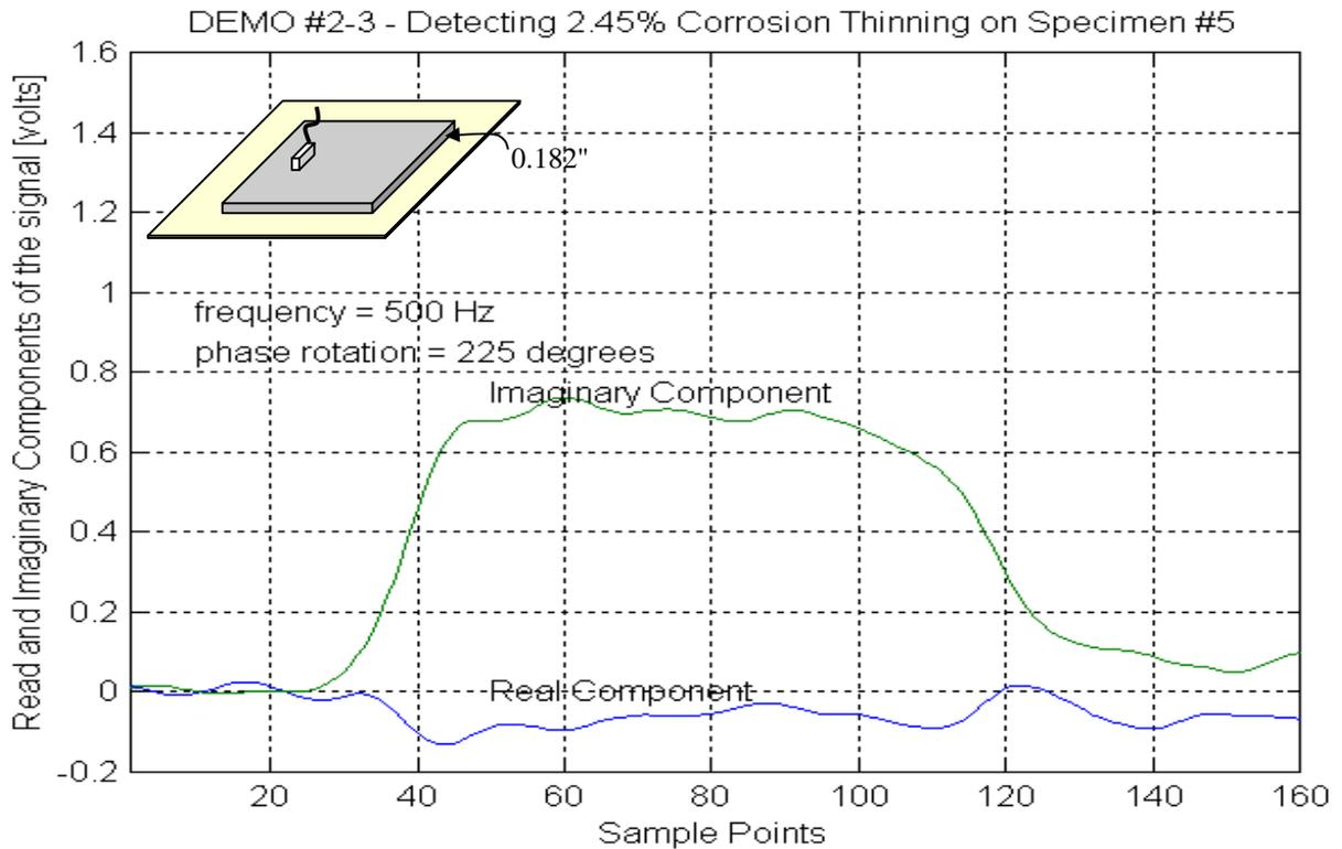
Figure 6. DEMO #2-3 - Thickness = 0.245", Corrosion Depth = 0.006", Relative Depth = 2.45 %
