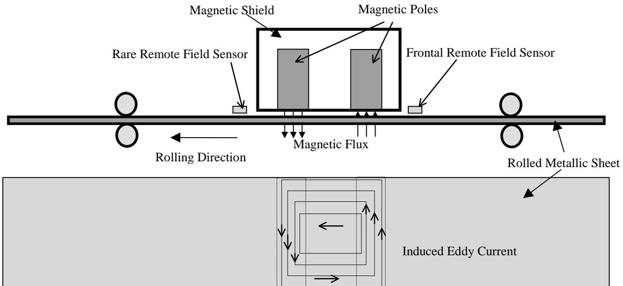
**Figure 3.** Fundamental idea showing the operating principle of the system
