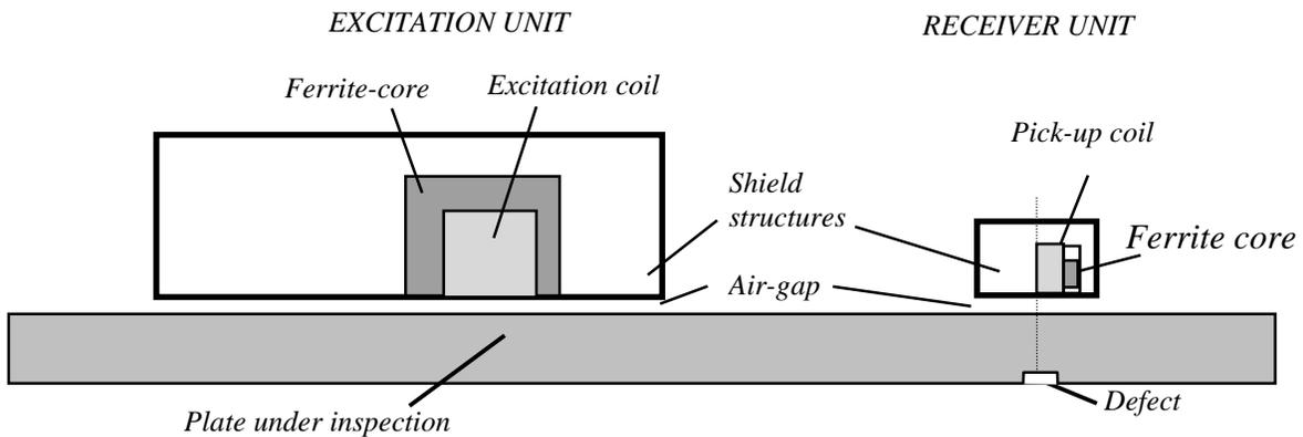
**Figure 2.** Prototype probe for inspecting metallic plates
