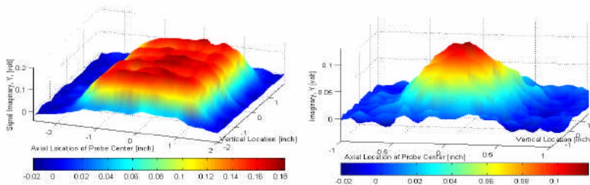
76 mm × 76 mm × 1 mm Flat-bottom corrosion 15.1 mm Below Surface
